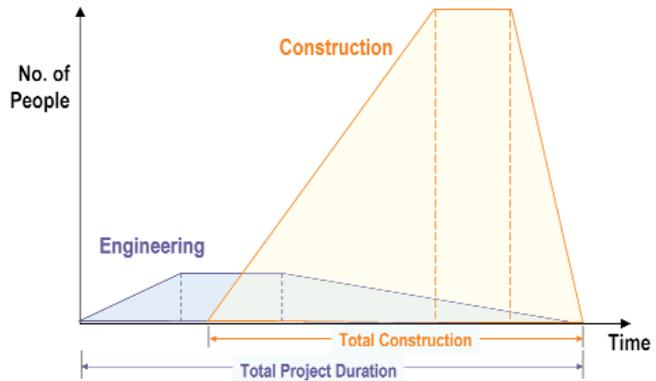
**Figure 2—Engineering and Construction Resource Profile Approximation**
